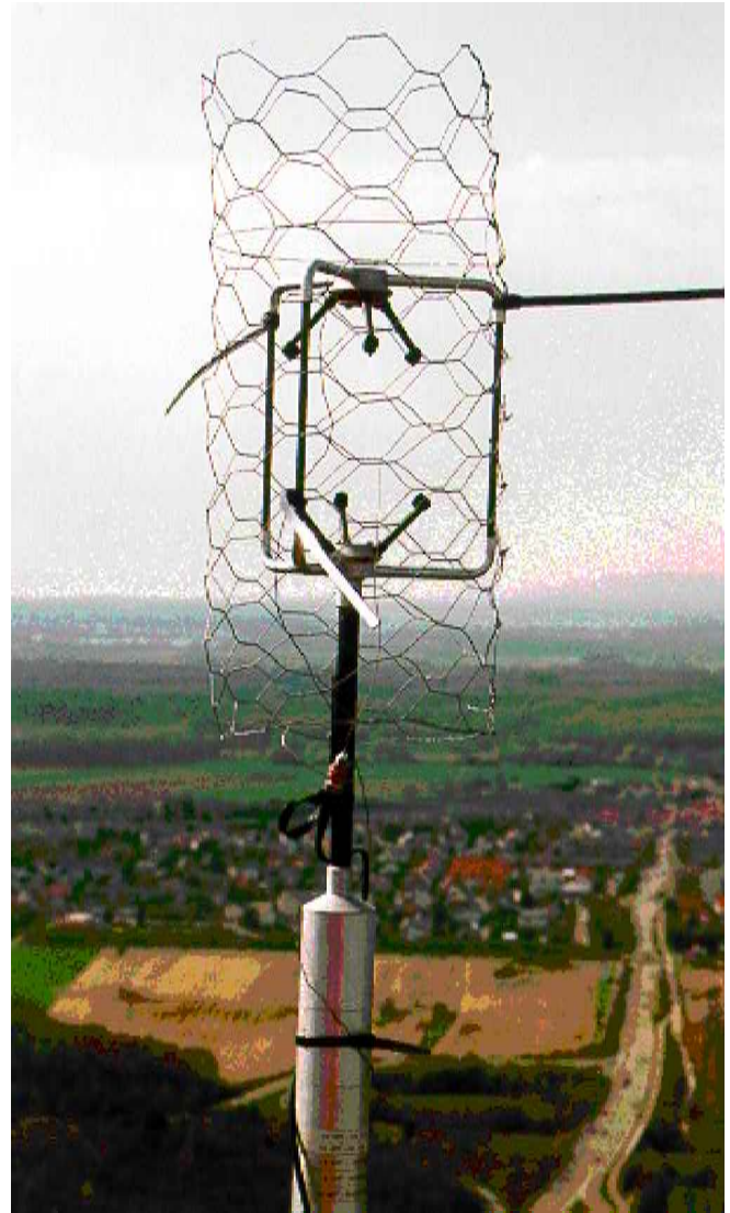
Figure 3: Gill ultrasonic anemometer with mesh wire.
